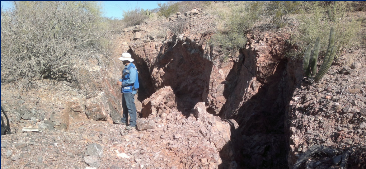
Old work 15 m long 5 m wide, work strike NW, structure strike N 75° W, dip 75° NE
