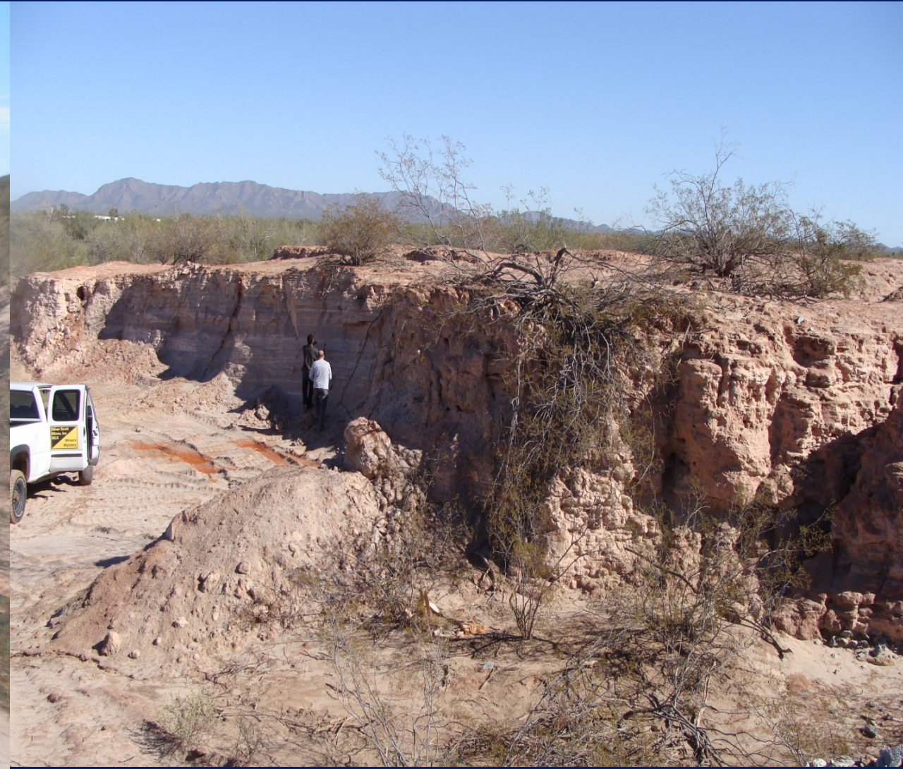
Old mill tailings pile on south side of Quitovac pueblo , where a sample contained 1.6 grams gold over a 2 m vertical continuous cut.
