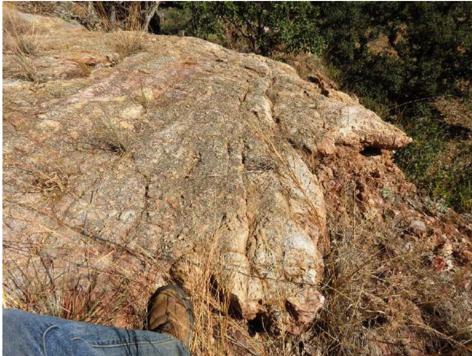
Figure 12. Low angle intensely silicified carapace breccia overlying earlier silicified breccia on upper surface of North Dome. View to south down dip from dome top.
