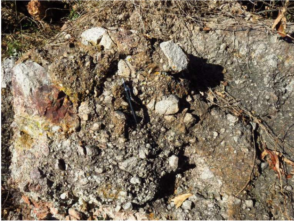
Figure 8. Intensely silicified breccia, South Dome area. Intense silicified felsic porphyry clasts in a silicified matrix. Similar breccias were observed near high grade mineralization in the El Salto and Mina Vieja portion of the Mulatos deposit.
